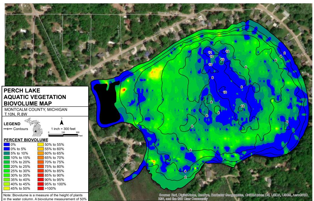
Note: Biovolume is a measure of the height of plants in the water column. A biovolume measurement of 50% indicates plants occupy one-half of the water column. Hydro-acoustic measurements conducted in September of 2019. Hydro-acoustic data processed by Navico.
